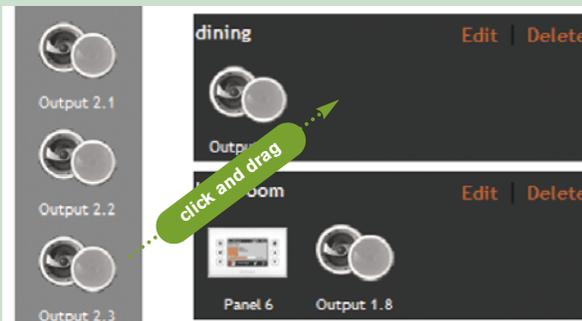
You will see that the speakers connected to the new IMA6 will be numbered 2.1, 2.2, etc.. (or 3.x, or 4.x depending on the number of IMAs connected). Simple drag these new speakers to the appropriate rooms and you are done.
