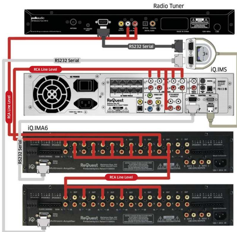
**Ensure that ALL devices are completely powered down before connecting.**
